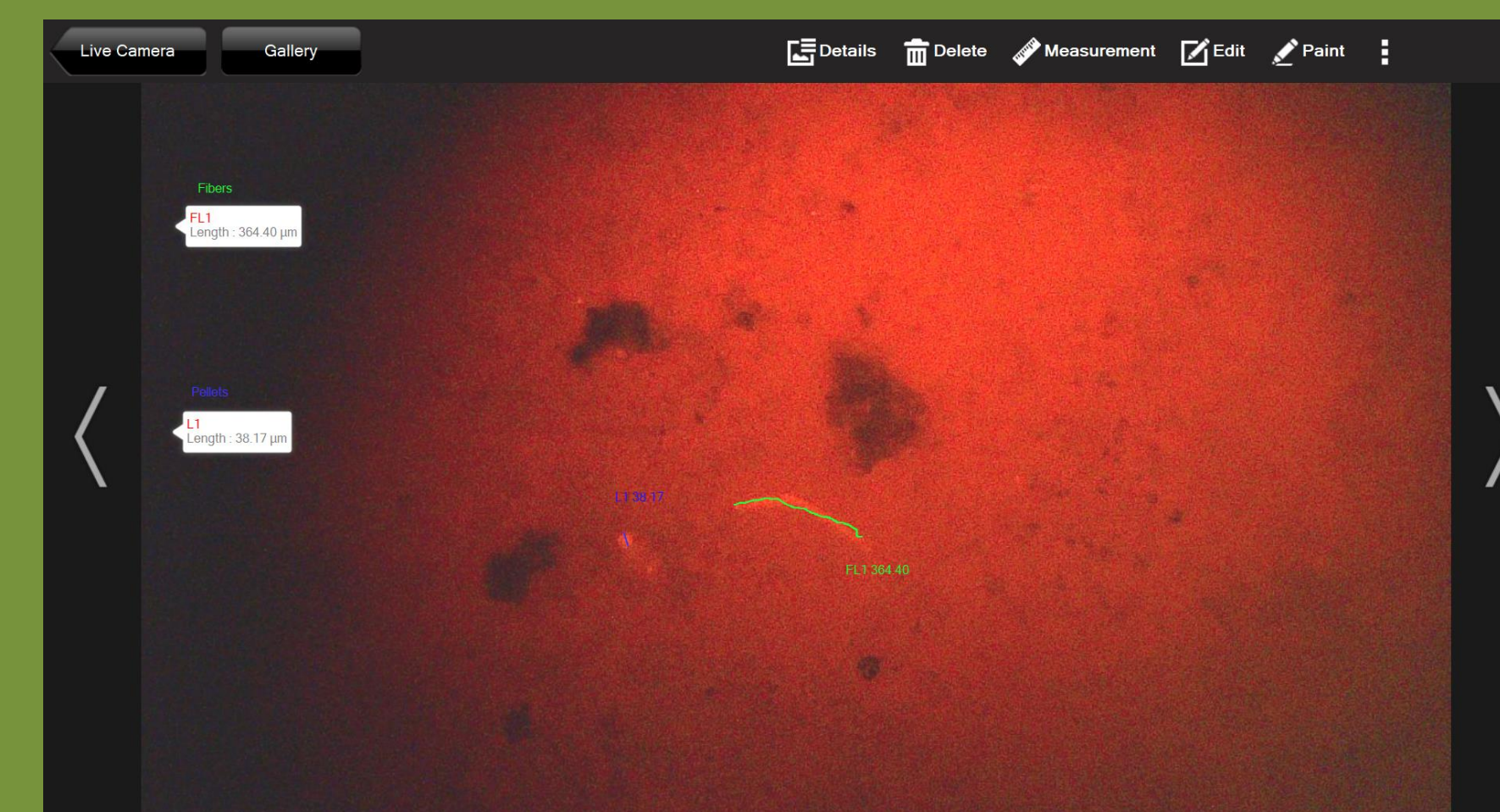
Blue nylon thread from Bethel sample 2 under fluorescent microscope
